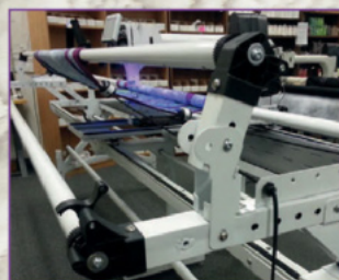
Batting access pivoting 2" tube allows for smoothing batting
